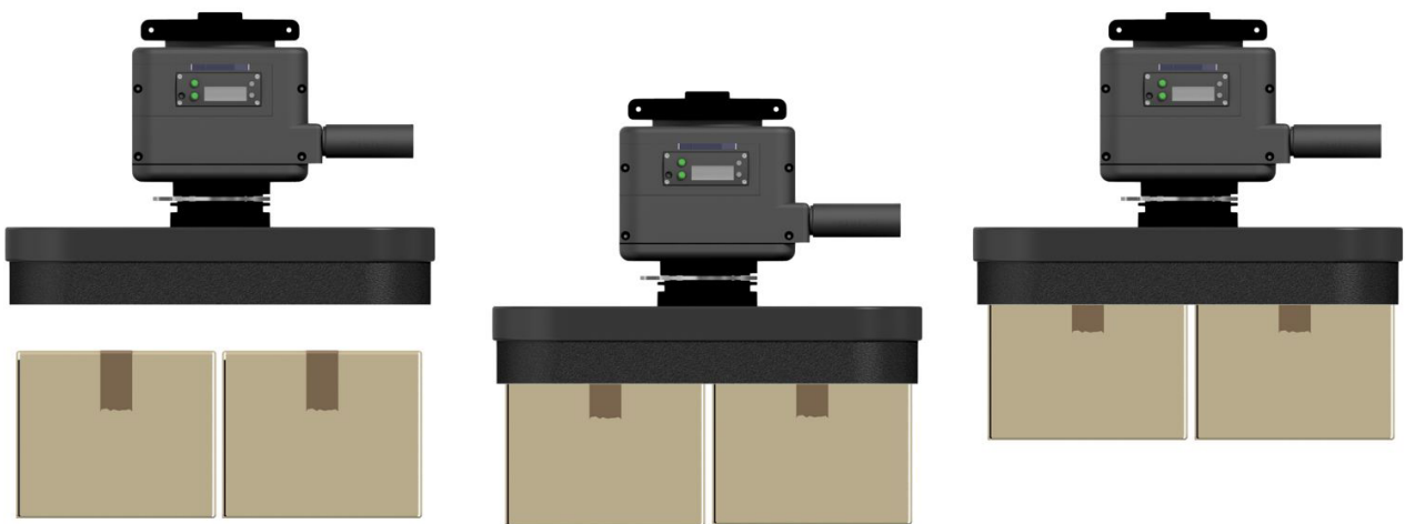
Figure 10 The working cycle of piCOBOT® L with foam gripper unit with flow reduction.
