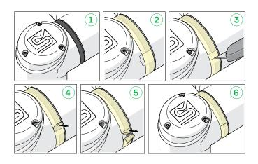
Attach the two spiral tube straps with straight tube connectors to the robot arm. Make sure that the straight tube connectors do not extend over any rotational joints of the robot.
