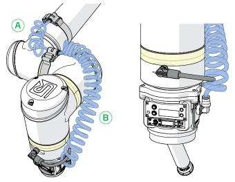
Cut the spiral tube leaving 4 to 5 loops (A) between the two straight tube connectors. Connect the new tube end to the straight tube connector on the second wrist of the robot.
