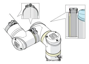
Attach the spiral tube from the EOAT to the straight tube connector on the third wrist of the robot. Make sure the tube is properly inserted into the straight tube connector.
