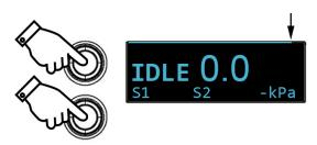
To enter the menus, press and hold "V" and "B" at the same time for 2 seconds. A small time-bar on the top of the display will gradually go from left to right until menus appear.
