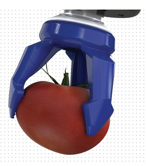
PIAB IS PROUD TO INTRODUCE the new soft gripping tool piSOFTGRIP®, developed especially with food industry automation in mind. The vacuum-based soft gripper will grip sensitive and lightweight objects of odd geometries and/or an unusual surface. Bin-picking of small irregularly shaped objects, such as toys, is another potential application.
